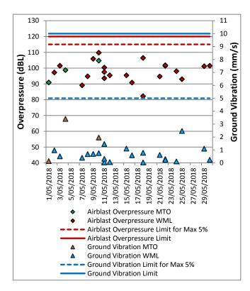
Figure 10: Bulga Village Blast Monitoring Results - May 2018
