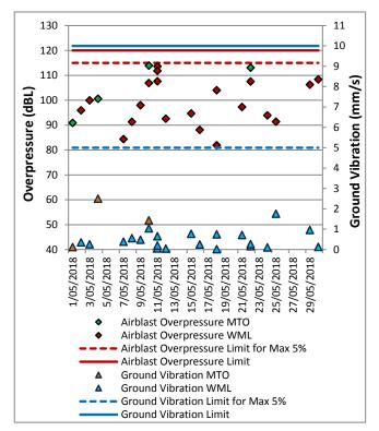
Figure 12: Wollemi Peak Road Blast Monitoring Results – May 2018
