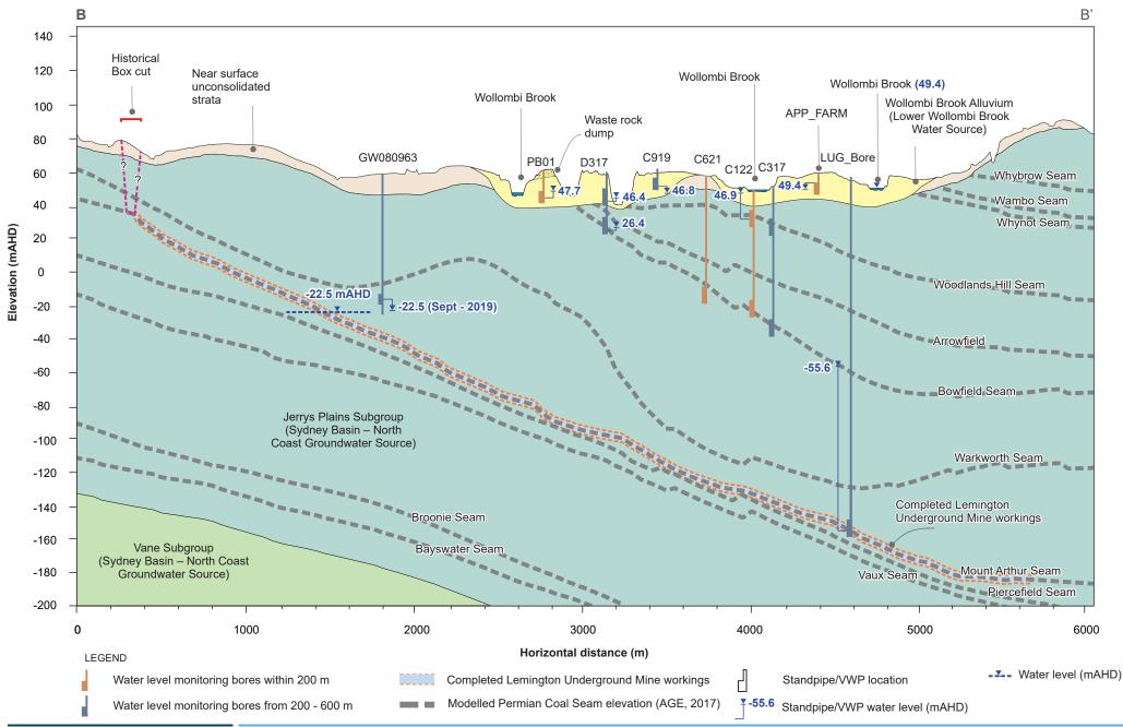
Conceptual hydrogeological cross section – B-B'
