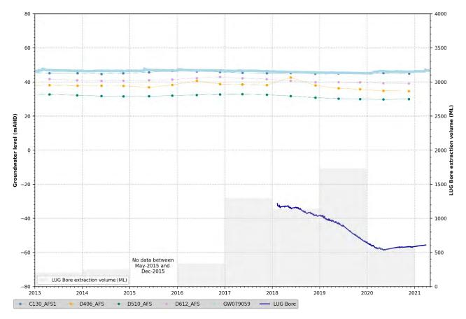
Figure 5.13 Groundwater levels Arrowfield coal seam
