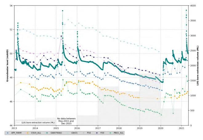
Figure 5.20 Wollombi Brook alluvium water levels compared to total annual extraction from LUG Bore
