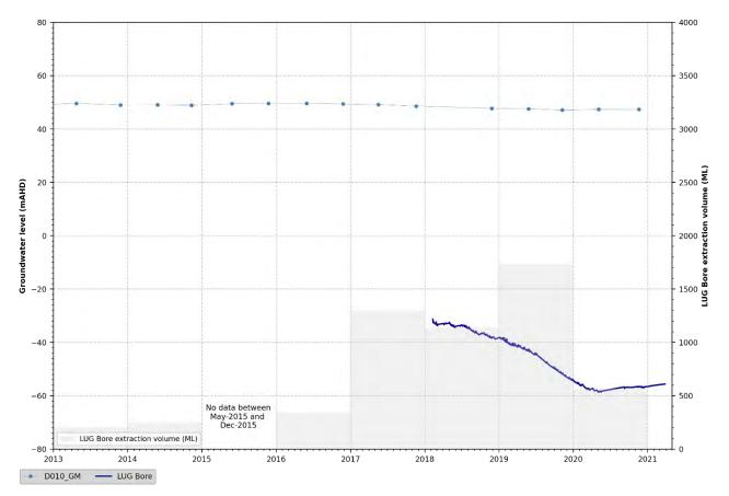
Figure 5.17 Groundwater levels Glen Munro coal seam
