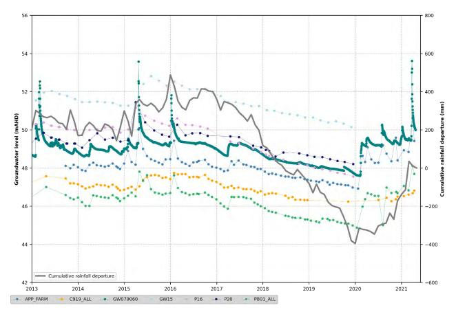
Figure 5.19 Wollombi Brook alluvium water levels compared to cumulative rainfall departure
