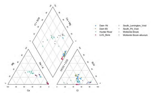
Figure 5.38 MTW main surface water stores, LUG Bore, surface drainages, and alluvium - Piper plot
