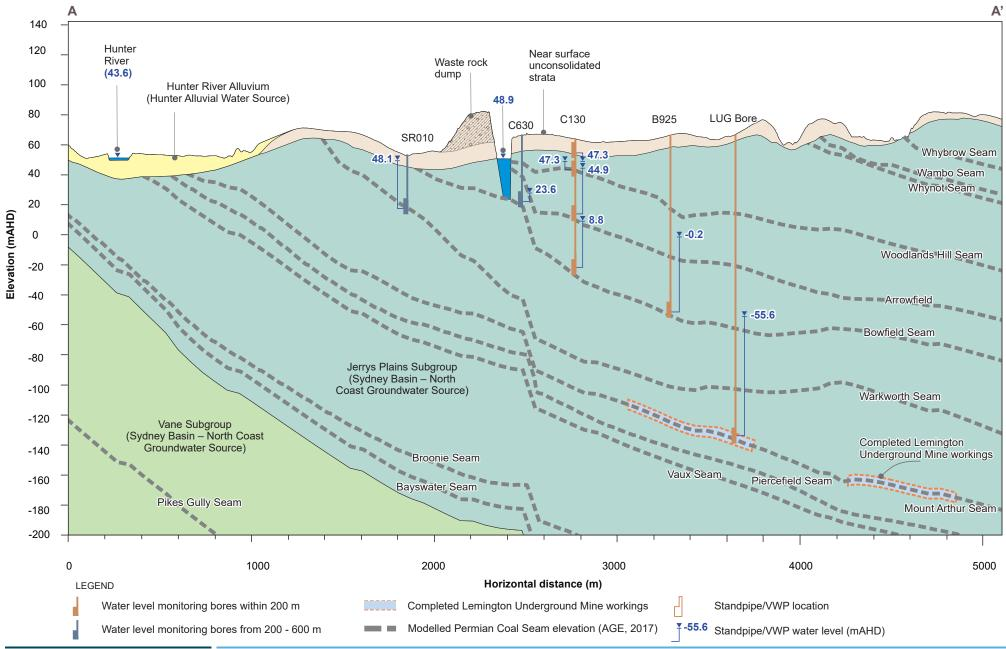
Conceptual hydrogeological cross section – A-A'
