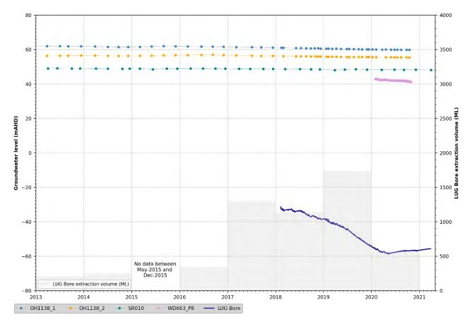
Figure 5.9 Groundwater levels Warkworth coal seam
